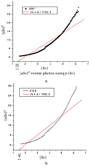
Fig. 7 –  $(\alpha hv)^2$ versus hv graphs for the samples sintered at 600 °C
