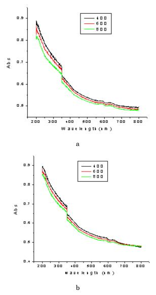
Fig. 6 – Absorbance versus wavelength graphs for CoMnO (a) and NiMnO (b) at  $400,\,600$  and  $800\,^{\circ}\text{C}$
